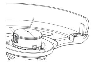
Put blade inside blade groove and fix the bolt.
