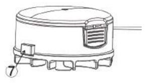
Press releasing button (7) and pull one end of grass trimming line at the same time. Loosen releasing button and repeat the step until the length of grass trimming line reaches the position of line cutting blade. If the length of grass trimming line is longer than the blade, excessive line will be cut off by blade. If the line is too long, take out of wire coil cover and rotate the wire coil anticlockwise until the required length is obtained.
