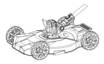
Lock the edge guide at the minimum length point. Insert the motor head into the guide(a) on the trimmer cart. Press the grass trimmer at an angle to the rear. The guard hood (b) will latch in the trimmer cart lock (c).
