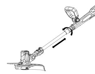
Rotate lock sleeve to the left based on the direction shown in the figure and stretch aluminum pipe to a proper position. Then fasten lock sleeve by rotating it to the right.
