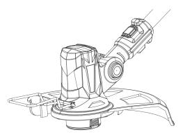
Fold protection steel as per Fig. A when grass trimmer is not used unfold it prior to grass or edge trimming.
