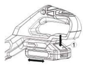
Press battery pack unlocking button (1) to take battery pack out of the machine. Push the battery pack that has been fully charged into the battery holder of grass trimmer softly and check if the pack has been installed firmly. The switch of this machine supports automatic back-locking function so as to avoid starting this machine by mistake. To start it, press (2) automatic lock button and switch (3) in order and release automatic lock button. Shut down the machine after loosening switch.
