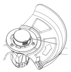
Align the two notches on shield with two columns on enclosure using a cross screwdriver according to the position shown in the figure above so as to fix the shield on enclosure.
