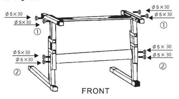
Connecting the screw hole position at the bottom of the piano body
