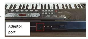
wrong socket is likely to cause electric hazard or damage.
