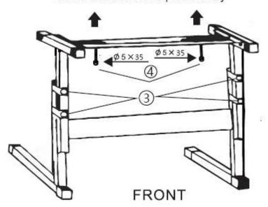
(3) Adjust the limit screw at the same time on the left and right sides to adjust the appropriate height
