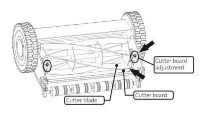
NOTE: Ensure both Cutter Board Adjustments (Part 17) have been adjusted to same corresponding height on each side of the assembly for safety and to ensure even cutting.
