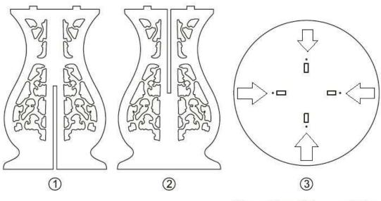
The position of the screw holes are indicated by arrows
