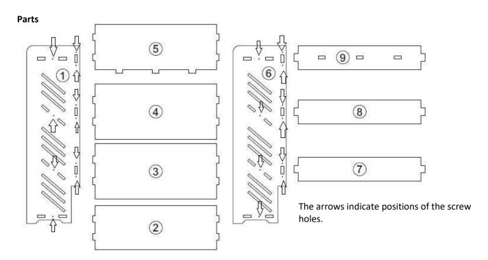
Parts are pushed together in the order as shown. After assembly, insert the screws (included) into to screw holes as indicated in Parts diagram for additional stability.
