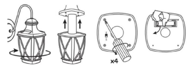
Untwist the bottom part of the lantern in a clockwise direction and pull down to access battery compartment. Undo the 4 screws and open the cover. Remove exhausted battery and replace with equivalent type. Reverse steps.
